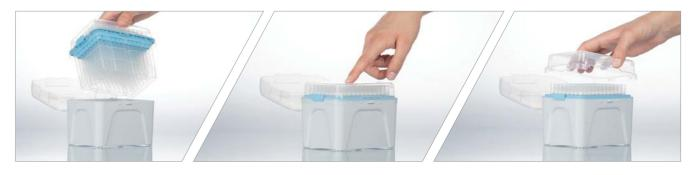
The complete SingleRefill is inserted into the box.
