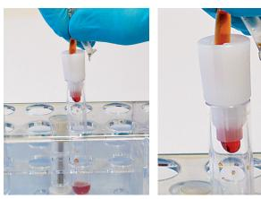
To empty the segment fold the tube and squeeze it. Dripping is avoided by releasing the pressure prior to removing the segment from the opener.
