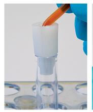
Hold tube segment opener in one hand. Insert tube segment at a slight angle (see Fig. a) and push forward without squeezing the tube.
