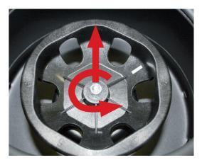
Losen and remove the rotor nut in the centre of the rotor using a 13 mm wrench (open counterclockwise direction).
