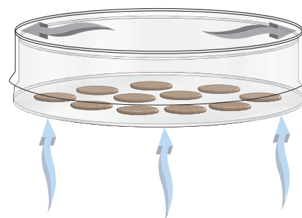
Fig. 4 No gas exchange possible in conventional cell culture vessels via the polystyrene or glass base
