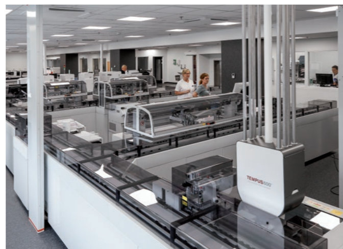
The Tempus600® connection module, as part of an automated one-touch handling system for samples tubes, provides a wide range of benefits, such as fewer work procedures, hands-free sample tube handling and generally faster and safer handling.
