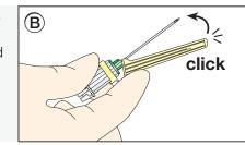
Alternatively, press down on the lower end cover and of the needle protector with your forefinger to cover and lock needle.
