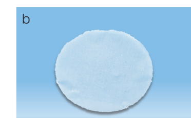
Detached PET membrane stays flat and does not curl.
