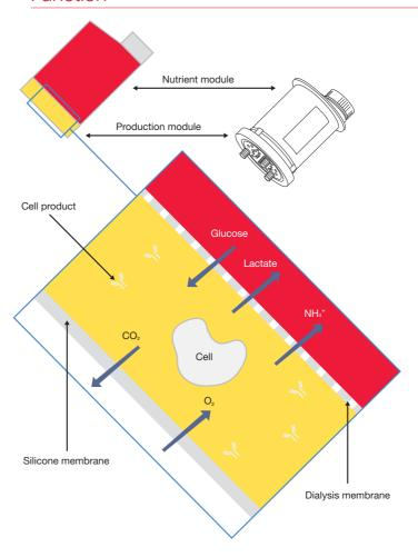
The miniPERM® bioreactor is a membrane-based two-compartment system.
